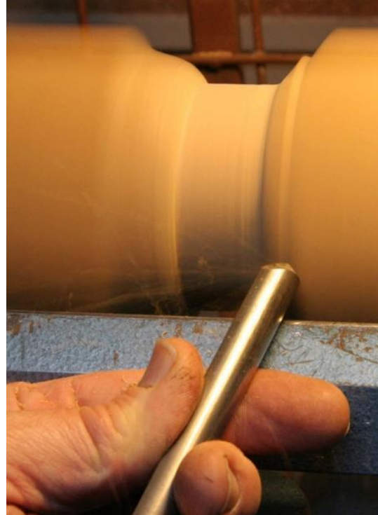
Cutting the Curved Shoulder.
