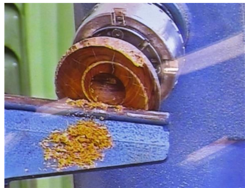
Lid with Spiral Catch and Large Tear Out on Outside
