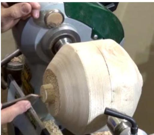
Theo remounted the blank in a horizontal orientation using previous spigot centres (see below).
