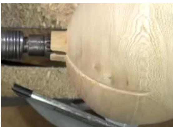
He refined the shape and reduced the spigots to almost nothing, doing the tailstock end first, and being careful not to damage the surface of the sphere.
