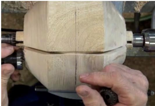
Theo advised that you can remove the waste down to the latest cut with a roughing tool, a 45 degree bowl gouge, a scraper, a spindle gouge, or a skew chisel as a negative raked scraper. He demonstrated all of these tool options. The objective was to remove the waste in 1 to 2mm cuts. He recommended looking at the horizon rather than the tool cutting to see the effect of the cuts you are making. He advised that you would get a better finish by cutting downhill rather than uphill.
