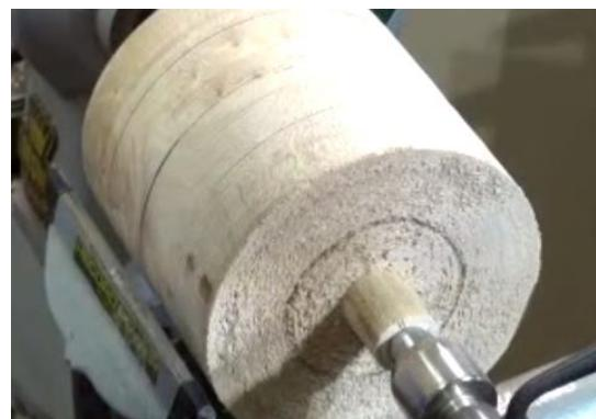
He then used a bowl gouge to remove waste from the shoulders of the blank. This is shown below.
