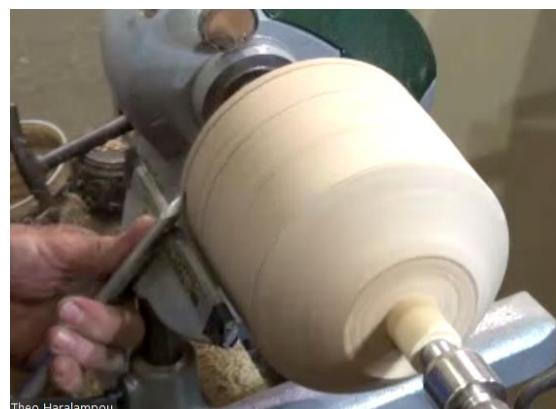
Using the indexing function of the lathe Theo determined the horizontal centre points on the round surface and marked them on the pencilled centre line. He marked them with a punch. He reduced the size of the spigots. Next, he removed the blank from the lathe, rotated it from the horizontal to the vertical orientation, and mounted it on the lathe using newly marked centres. The result is shown below. Theo stressed the need to be accurate and careful when centring the blank.
