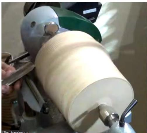
Theo had the lathe running at 700 rpm. When the gap between the blank and the toolrest widened he stopped the lathe, moved the toolrest closer, tightened the tailstock, and increased the speed to 900 rpm. When he was satisfied with the blank Theo marked the
