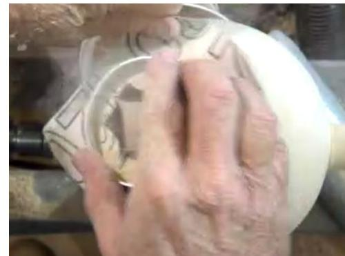
Theo removed the spigots off the lathe using a small fine tooth saw. The following image shows Theo holding the completed sphere.
