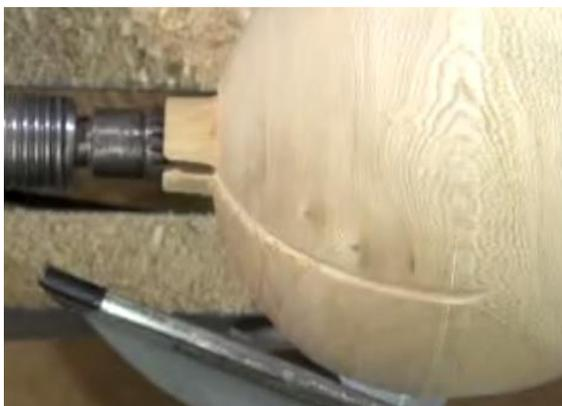
He refined the shape and reduced the spigots to almost nothing, doing the tailstock end first, and being careful not to damage the surface of the sphere.
